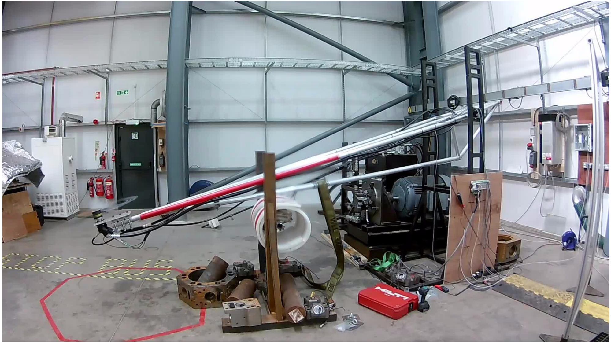
Video of full-size rotor test rig (1.5m diameter) – capable of 100kg thrust
